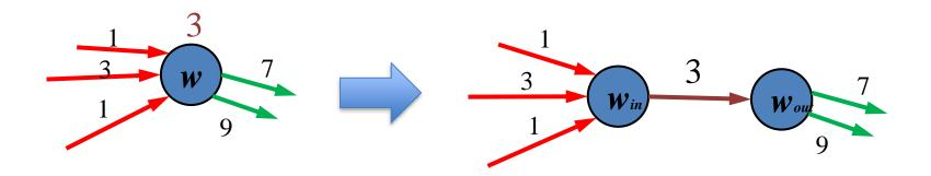
Fast approach: Transform the capacity on vertices to capacities on edges. For every vertex w, create two new vertices  $w_{in}$ ,  $w_{out}$  and connect all incoming edges of w to  $w_{in}$  and all outgoing edges to  $w_{out}$ .
