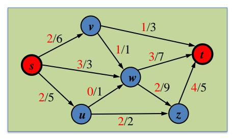
Augmenting path: Path from **s** to **t** with positive residual capacities.
