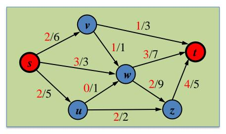
$s \rightarrow v \rightarrow t$ : 2 units of flow can be pushed (min over residual capacities).
